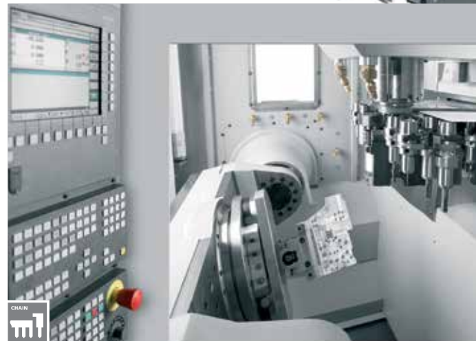
Automatic tool change with the pick-up method as fast as 0.9 s (48 tool places).
