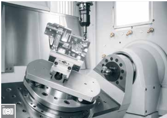
2-axis swivel rotary table for economical complete machining with five simultaneously controlled axes.
